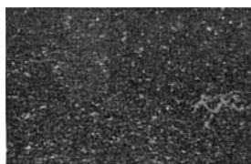
Figure 5. PBLG+MBBA aggregates (light areas) floating in oriented nematic (black between crossed polaroids). The small aggregates diffuse through the nematic to form large aggregates (magnification 1000\times ).
